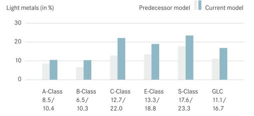
The lower percentage of **steels and ferrous materials** and the increasing share of **light metals** illustrate the new approach now being taken with our vehicle architectures, which in some cases has led to a substantial weight reduction for the entire vehicle.
