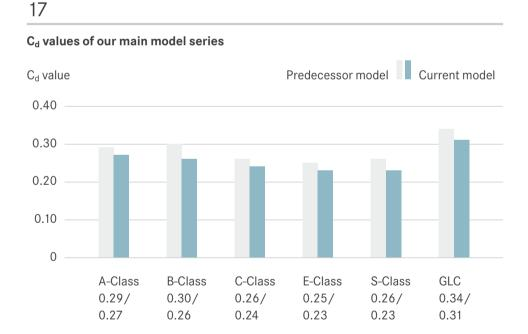
C<sub>d</sub> (drag coefficient): Figure used to quantify the resistance of an object in a fluid environment, such as air or water. A reduction of a vehicle's C<sub>d</sub> value by 0.01 lowers fuel consumption by approximately 0.1 I/100km.
