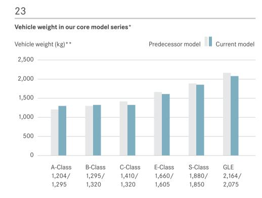
The trend toward increasing weight due to more features and additional safety equipment has been reversed in the new series thanks to intensive weight management.
