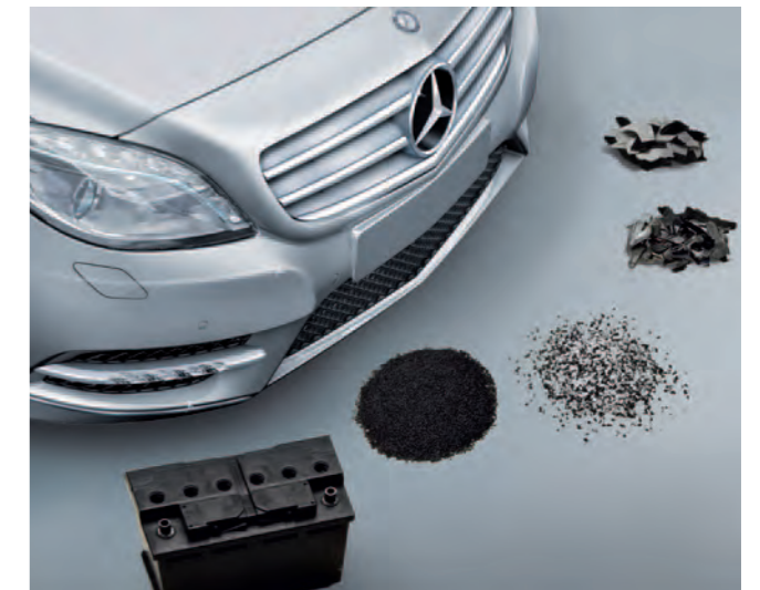
Use of secondary raw materials, taking the wheel arch lining as an example (as here in the current B-Class)
