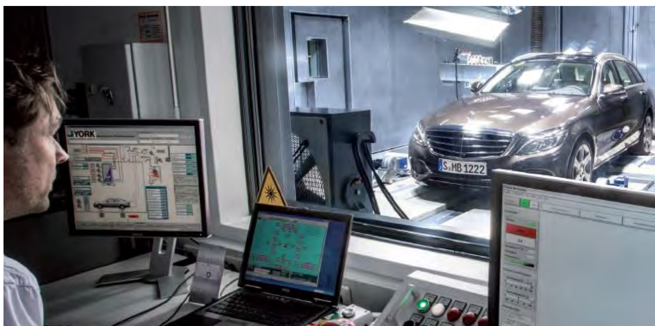
Figure 3-1: Test chamber to measure car cabin emissions
