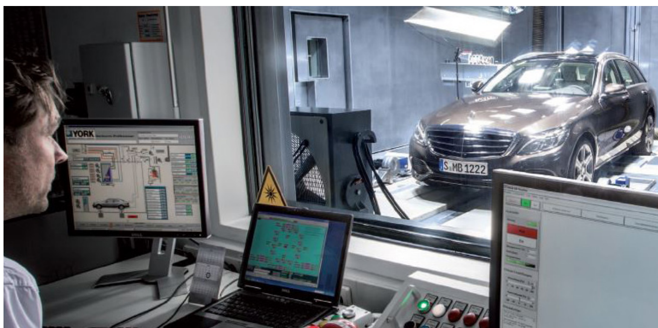
Figure 3-1: Test chamber to measure car cabin emissions
