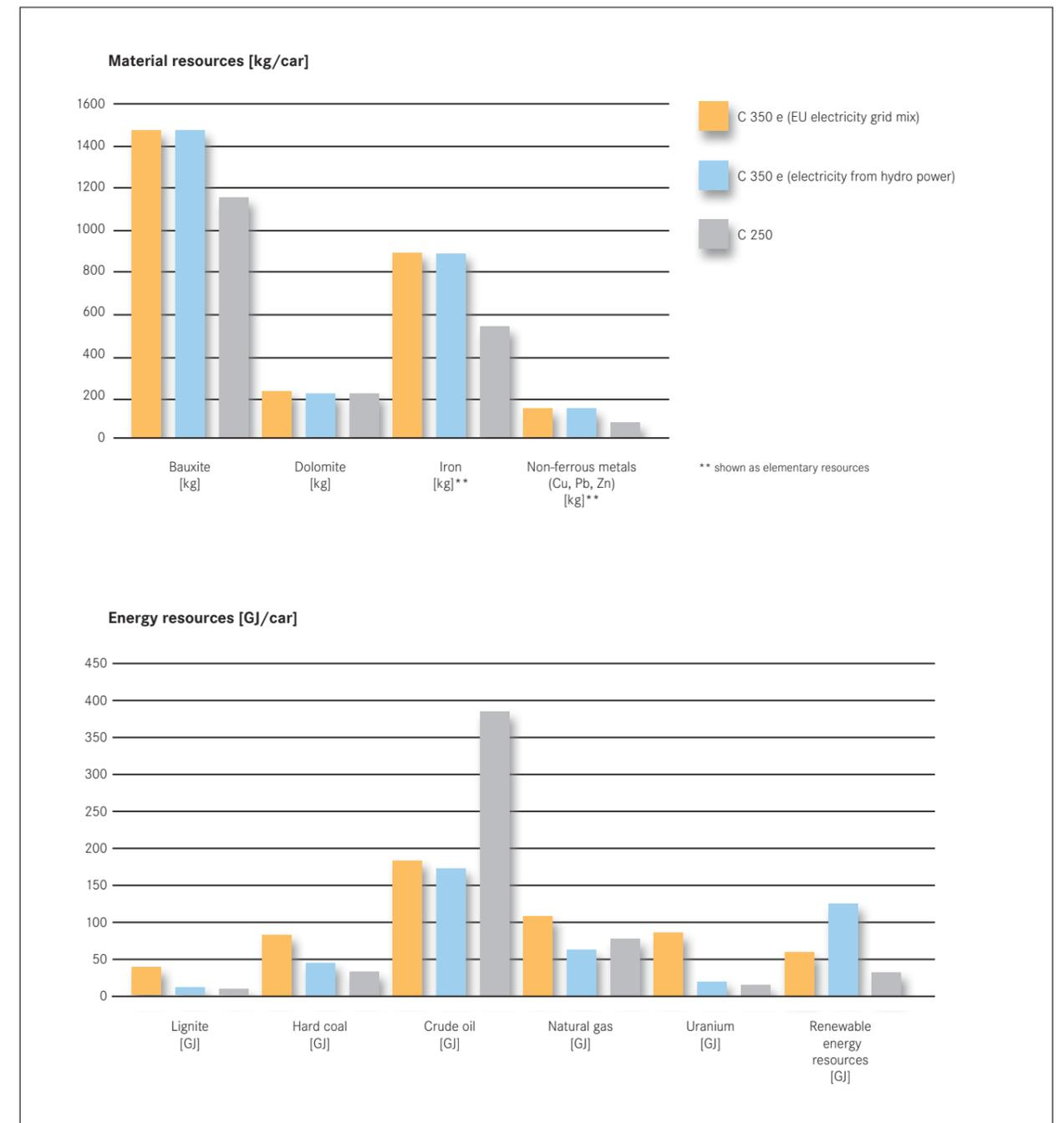
Figure 2-12: Consumption of selected material and energy resources compared to the predecessor C 250 [unit/car]
