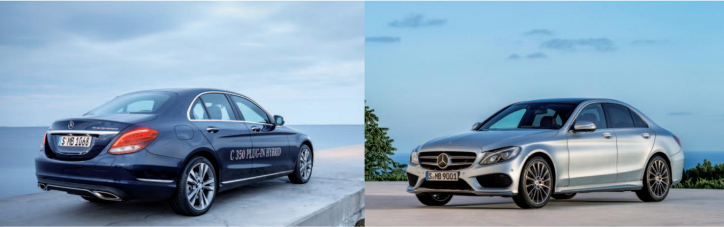
The plug-in hybrid model in the current C-Class, the C 350 e, combines a 60 kW electric motor and an externally rechargeable battery with a four-cylinder petrol engine displacing just under two litres.
