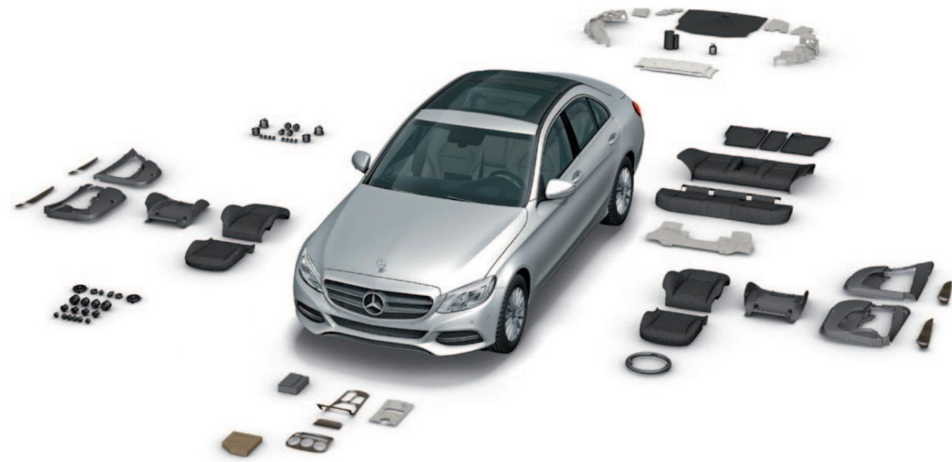
In the new C-Class, a total of 76 components with an overall weight of 26.3 kilograms are made using natural materials. The total weight of components manufactured with the use of renewable raw materials has thus increased by 55 percent compared with the preceding model. Fig. 2-16 shows the components in the new C-Class which are produced using renewable raw materials.
