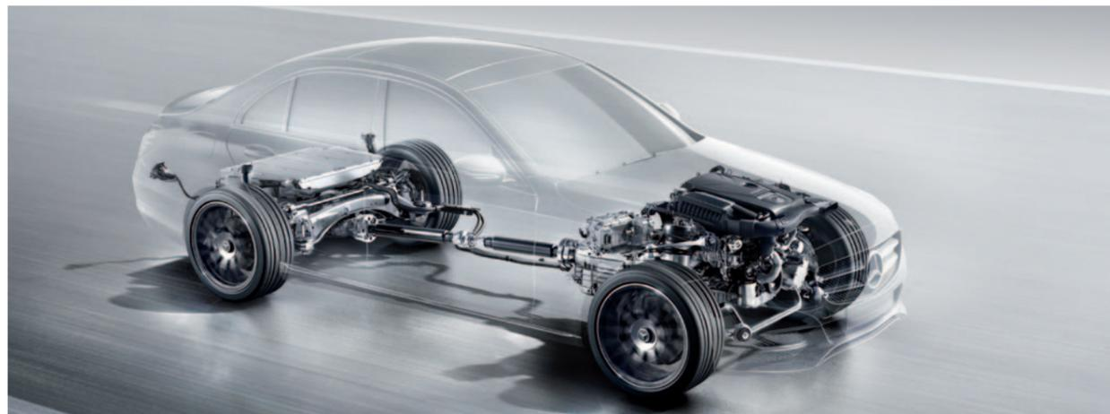
The plug-in hybrid technology can be integrated into the structure of the C-Class without any modifications, as the second-generation hybrid transmission is based on the 7G-TRONIC PLUS automatic transmission. Despite the space taken up by the battery, the C 350 e Saloon has a boot capacity of 335 litres.
