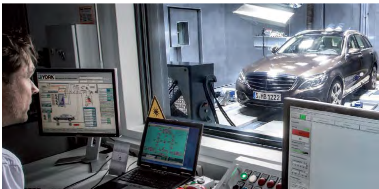
Figure 3-1: Test chamber to measure car cabin emissions
