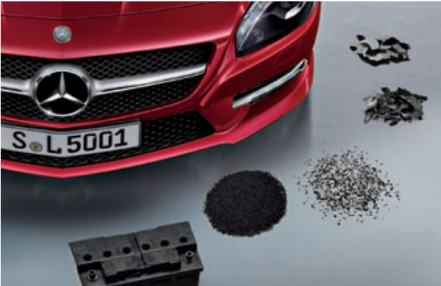
Figure 2-15: Use of secondary raw materials, taking the wheel arch lining as an example.
