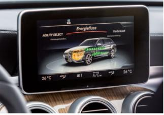
Working in the background, the intelligent engine management system in the C 350 e selects the ideal combination of combustion engine and electric motor automatically. Then there are innovative functions such as the route-based operating strategy or the haptic accelerator pedal which can help the driver to drive economically.
