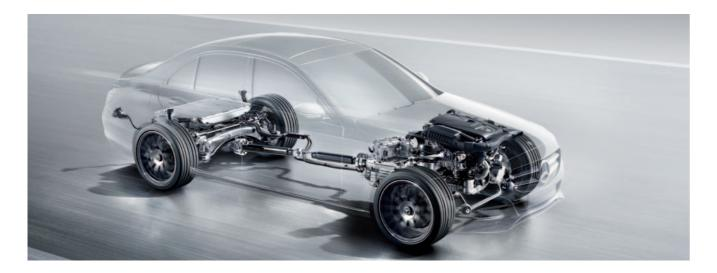
The plug-in hybrid technology can be integrated into the structure of the C-Class without any modifications, as the second-generation hybrid transmission is based on the 7G-TRONIC PLUS automatic transmission. Despite the space taken up by the battery, the C 350 e Saloon has a boot capacity of 335 litres.
