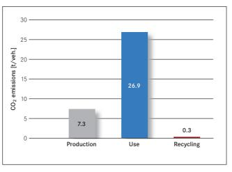
Figure 2-3: Overall carbon dioxide emissionen (CO<sub>2</sub>) in tonnes
