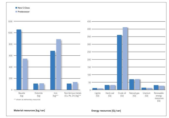
Figure 2-9: Consumption of selected material and energy resources by the new C 180 compared with the predecessor from 2013 [unit/car]
