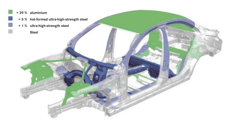
Mercedes-Benz achieves this feat of lightweight construction by various measures, including a completely new structural design and the use of an unusually high proportion of aluminium for a high-volume series. Compared with the successful predecessor, the aluminium content has increased from less than 10 percent to almost 50 percent.
