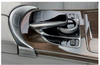
All the functions of the head unit can be controlled simply and intuitively from the touchpad, using fingertip gestures. The air-conditioning system of the new C-Class offers tunnel recognition using the satellite navigation system, whereby the air recirculation flap is automatically closed when the vehicle enters a tunnel and re-opened when it emerges.
