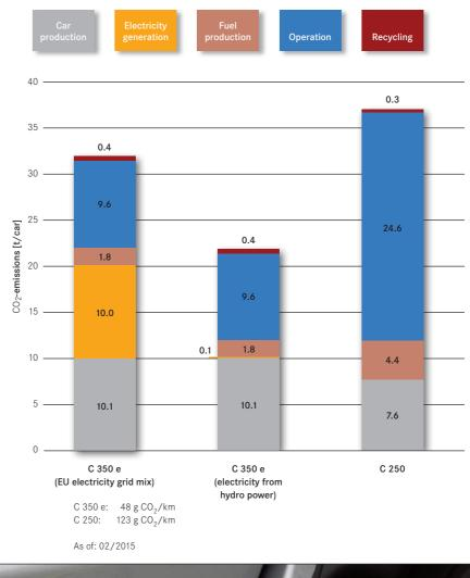
Figure 2-10: Comparison between th of the C 350 e and the C 250 [t/car]
