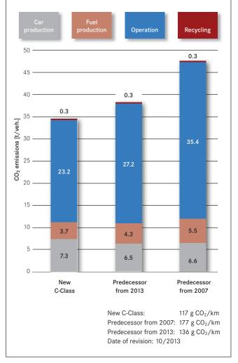
Figure 2-7: Carbon dioxide emissions of the C 180 in comparison to its predecessor [t/car].
