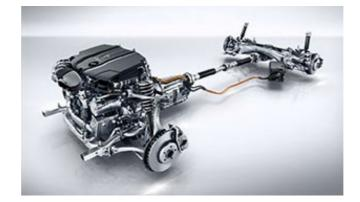
Mercedes-Benz has transferred the BlueDIRECT technology from the V6 and V8 engines to the four-cylinder engine. The direct injection system with spray-guided combustion, first introduced into passenger car series production by Mercedes-Benz, employs an electronically controlled precision multiple injection process.
