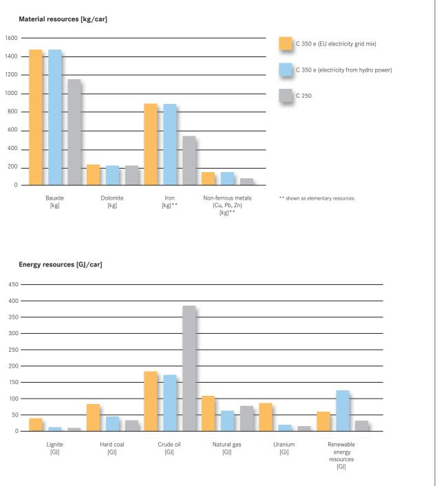
Figure 2-12: Consumption of selected material and energy resources compared to the predecessor C 250 [unit/car]
