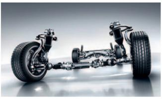
The suspension offers exemplary springing and road roar and tyre vibration characteristics, combined at the same time with outstanding dynamic handling. In addition, the new C-Class is the first vehicle in its segment that can be fitted with air suspension (AIRMATIC) at the front and rear axles.
