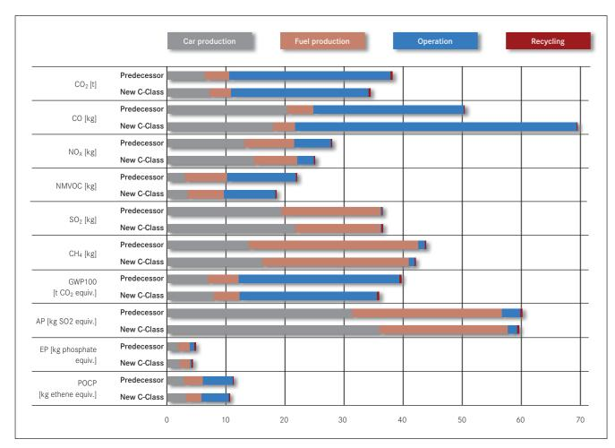
Figure 2-8: Selected result parameters for the C 180 compared with its predecessor from 2013 [unit/car]
