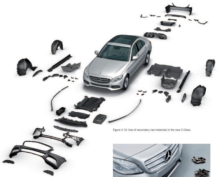
In the new C-Class, 52 components with an overall weight of 49.3 kilograms can be manufactured partly from high-quality recycled plastics. The weight of secondary raw material components could thus be increased by 23 percent compared with the preceding model. Typical areas of use are wheel arch linings and underbody panels, which consist for the most part of polypropylene. Fig. 2-15 shows the components for which the use of secondary raw materials is approved.
