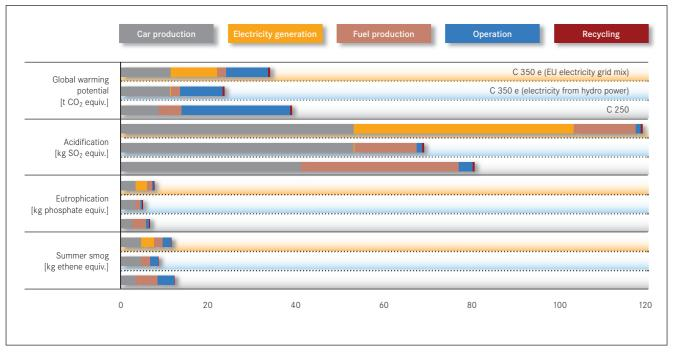
Figure 2-11: Selected result parameters for the C 350 e compared to the C 250 [unit/car]
