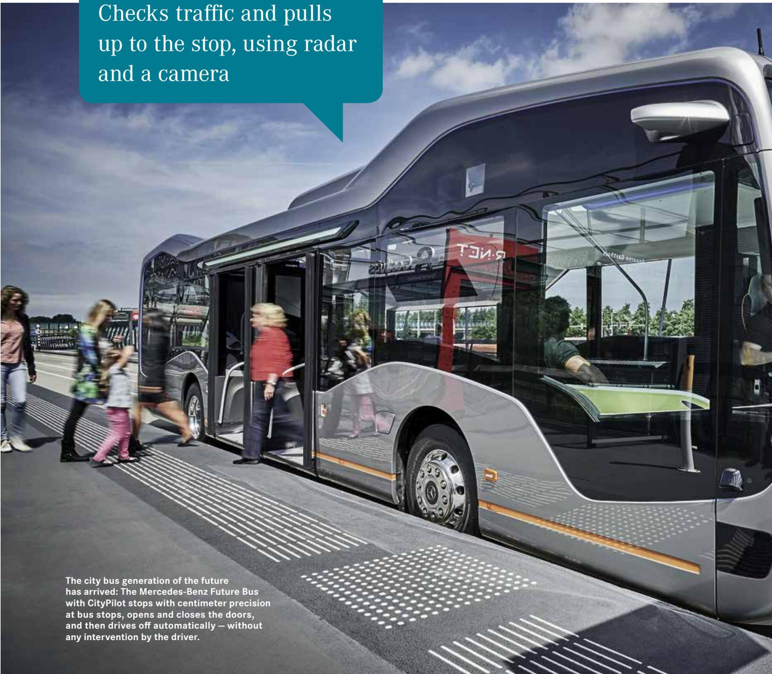
The city bus generation of the future has arrived: The Mercedes-Benz Future Bus with CityPilot stops with centimeter precision at bus stops, opens and closes the doors, and then drives off automatically – without any intervention by the driver.
