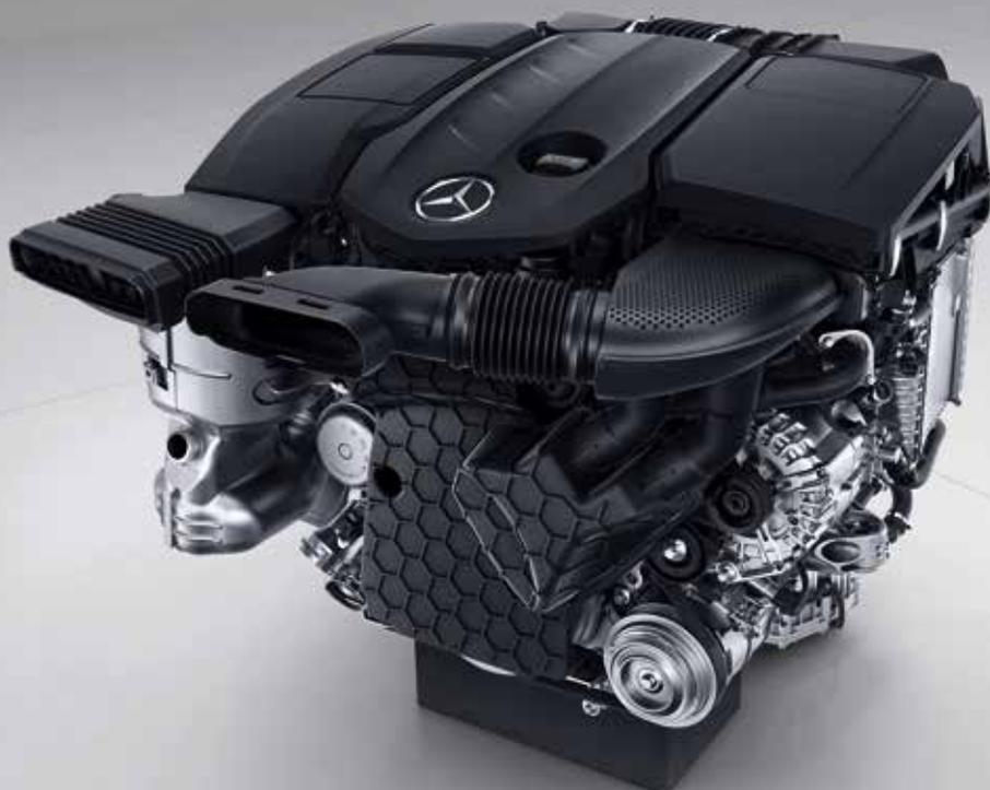
More fuel-efficient, lighter and more compact: the new four-cylinder diesel OM 654 from Mercedes-Benz starts a new engine family.
