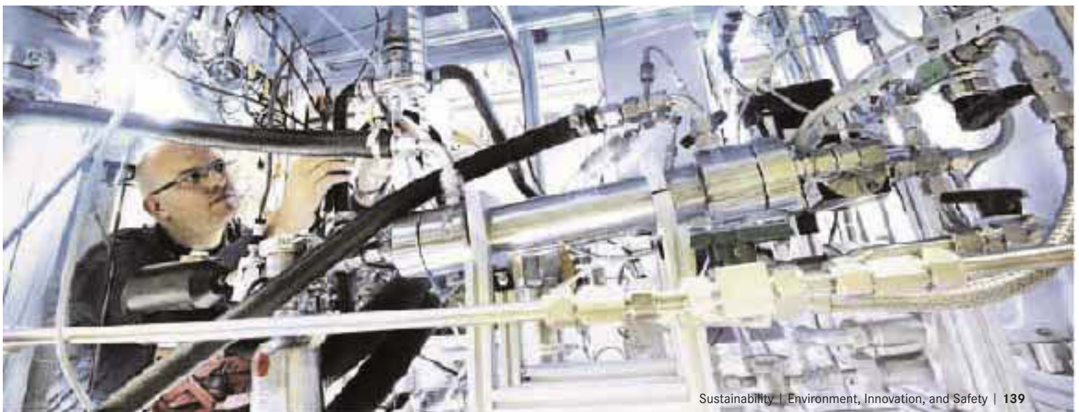
Testbench for electric drive with fuel cells.
