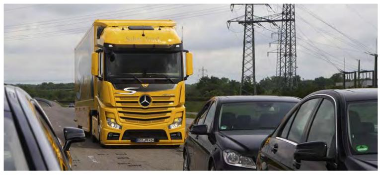
The new "Active Brake Assist 3" now independently applies the full brakes if a stationary object is detected ahead.
