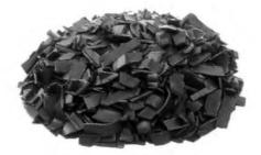
Painted polycarbonate car bumpers are ground in preparation for qualified processing. The high-grade stripping of the polycarbonate chips results in a plastic that is reprocessed into high-grade recycled materials.
