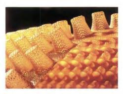
A three-dimensional braid of plastic fibers is a potential material for light-gauge construction. The highly ductile burled pattern is an ideal base structure for the production of light-weight but very solid parts, even with complicated shapes.
