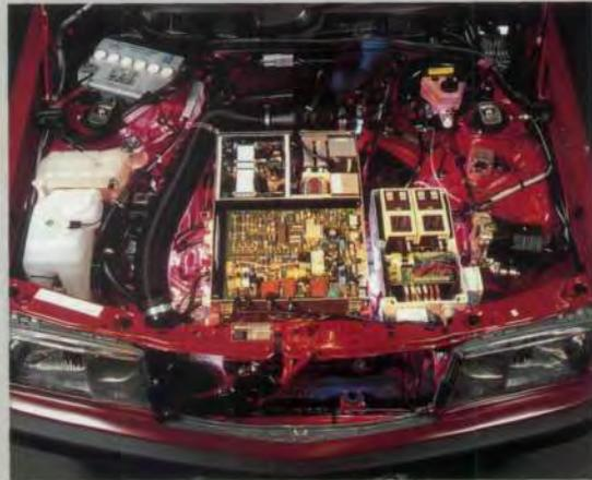
View under the engine hood of an electrically powered car from the Daimler-Benz Research division.
