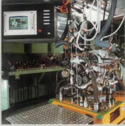
Fully automatic final testing of twelve-cylinder engines at Mercedes-Benz AG's plant in Stuttgart-Untertürkheim.
