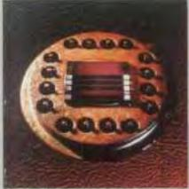
Chemical semiconductor sensor for direct electronic measuring of pollutant and ionic concentrations in liquid and gaseous substances.
