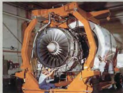
Preparation of a V 2500 engine for testing.
