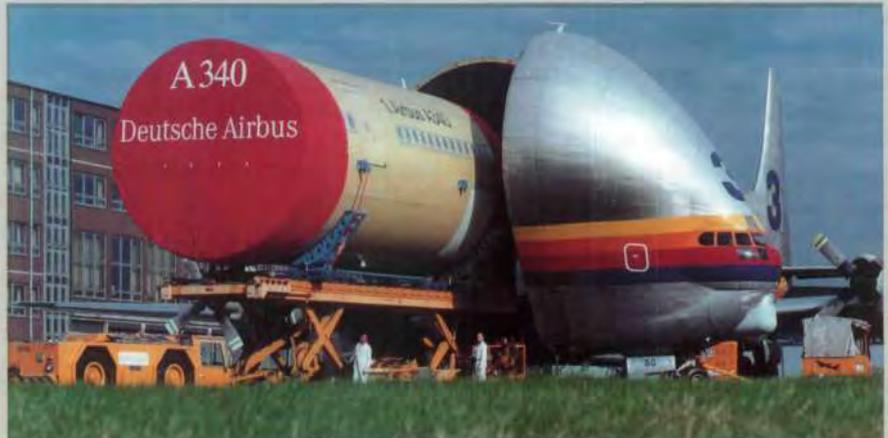
Loading the first front fuselage segment for the new A 340 Airbus into a "Super Guppy" transport aircraft.
