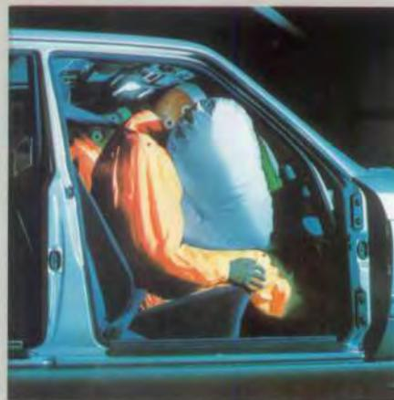
A special airbag for the front passenger complements the driver airbag.
