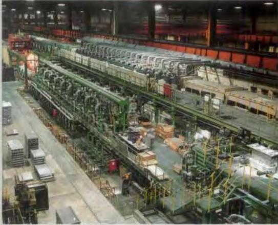
Automated electrolytic coil-coating plant for sheet steel.
