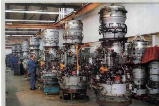
Assembly line for the Tyne turboshaft engines.
