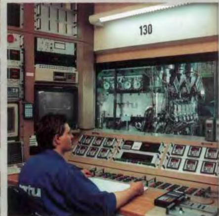
The new 595 diesel engine series on the test bench.
