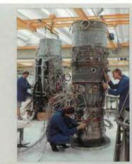
Highly-qualified staff are required for the assembly of modern aero-engines, e.g. the EJ 200.
