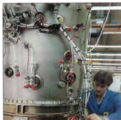
RB 199 engines for the Tornado are assembled in vertical position. Hydraulic lift platforms allow working at the ergonomically favorable level.
