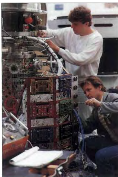
Connecting of measuring cables to a test engine.
