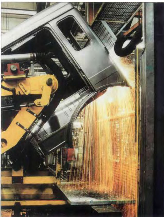
Shielded arc welding in cab shell manufacture (Wörth plant).
