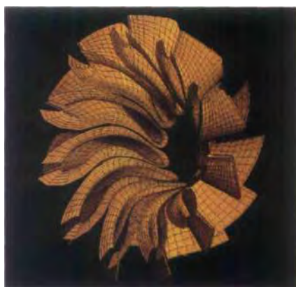
Milling pathways for NC manufacture of a turbocharger-turbine wheel: the turbine wheels are developed via a closed data transfer, which extends from the aerodynamic design right up to manufacture.
