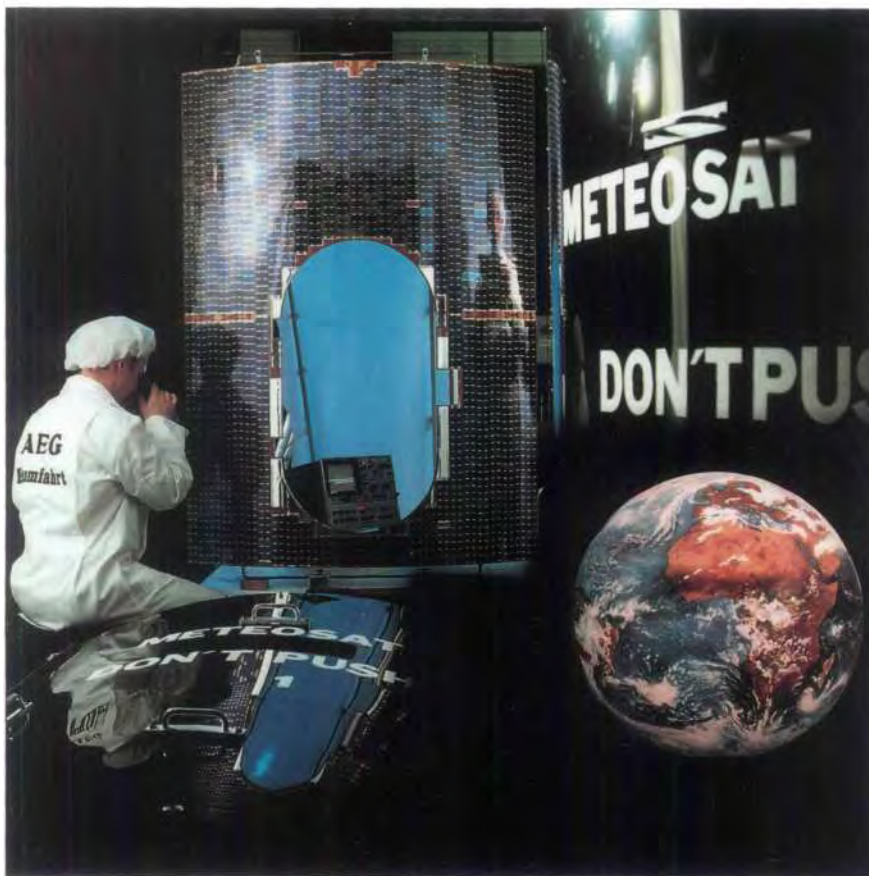
Measurement of a structural panel for the METEOSAT meteorological satellite in Wedel near Hamburg. AEG built the complete solar generator for the satellite. Roughly 33,000 solar cells sized 19.8 x 39.6 mm were installed on the METEOSAT.
