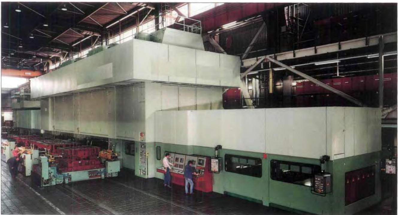
Procurement in the capital goods sector: this ultra-modern gang press for large parts in the Bremen plant was developed in cooperation with a specialist in the plant and equipment industry.
