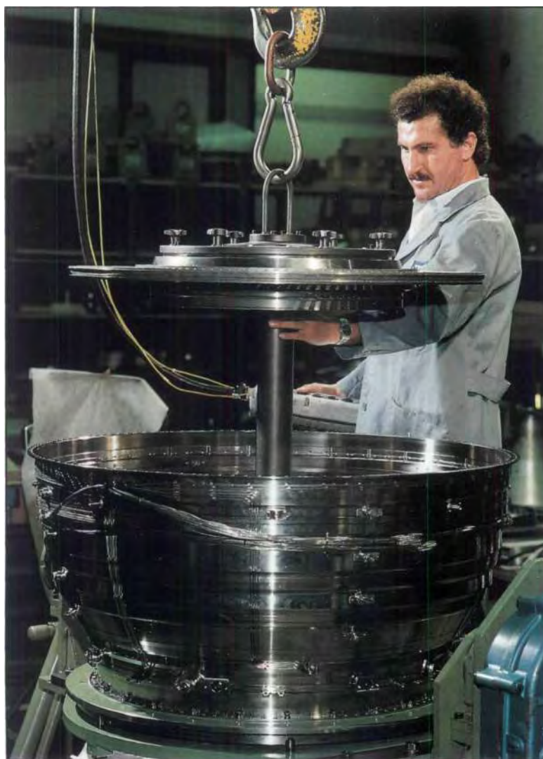
Assembly of a low-pressure turbine from MTU for the jet engine of a modern commercial aircraft.
