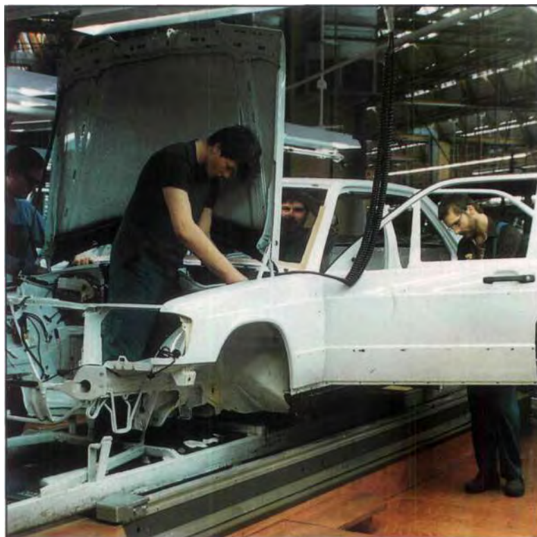
Greater personal responsibility for one's work: assembly teams install the complete electric equipment in the stationary vehicle.
