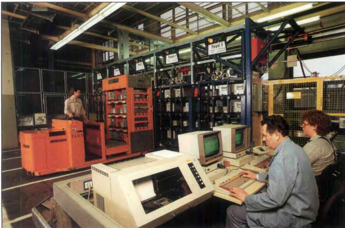
Rationalized flow of materials in the new, fully automated high stacker for small parts in the Untertuerkheim plant.
