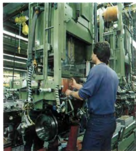
Precision work during the valve adjustment of the 190/190 E engines in the Untertuerkheim plant.
