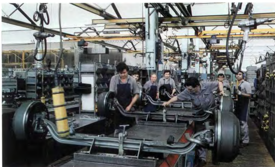
Assembly of front axles for trucks at Mercedes-Benz Argentina.
