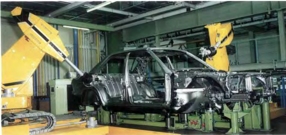
Body Quality Control Station: using two eight-axled industrial robots, programmable for different models, 500 test points are checked for proper tolerance.
