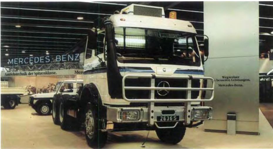
For world-wide application, Mercedes-Benz developed the 2636 S/6 x 4. Long-haul tractor equipped with a naturally aspirated 261 kw (355 hp) engine.
