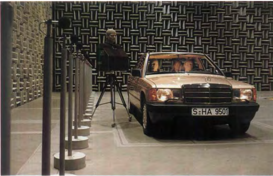
Unparalleled in the world to date, the unique procedure for isolating and measuring external noises. The Daimler-Benz test facility - jointly developed with the Technical University of Aachen - permits the objective comparison of noise levels and thus the purposeful reduction of noise sources.
