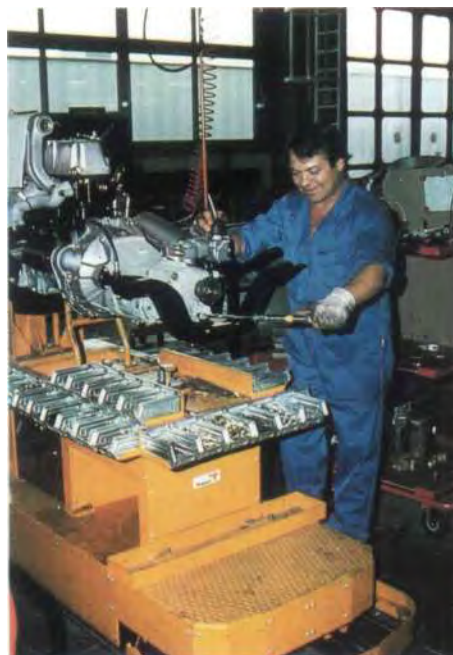
Single work stations permit employees to work independently of line speed and according to their own abilities. Unrealistic bodystress positions are avoided with specially created work stations.
