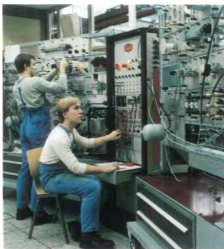
Example of practical application of professionally-oriented job training: construction and testing of electric-hydraulic circuits.
