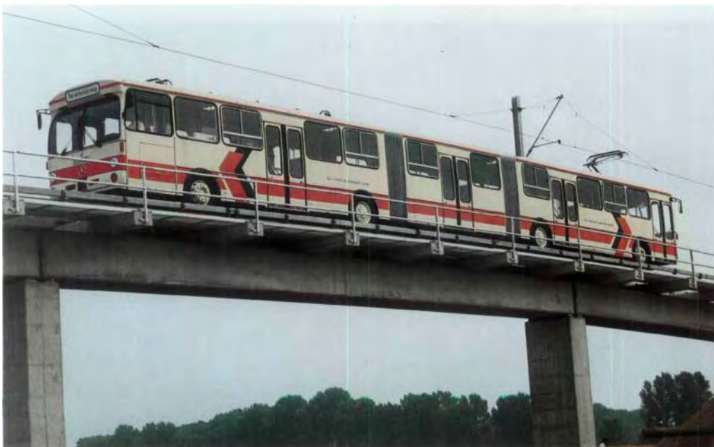
The high-capacity and electrically powered Mercedes-Benz O-Way is fed by overhead cable, at the Rastatt test track.
