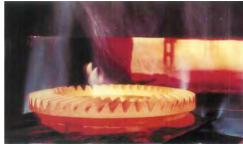
Example of modern manufacturing technology in the Kassel plant: Case hardening of ring-gears in continuous push-through oven.
