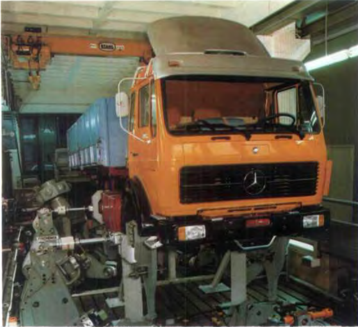
The computer-operated vibration test stand for commercial vehicles eliminates the necessity of durability on test tracks.
