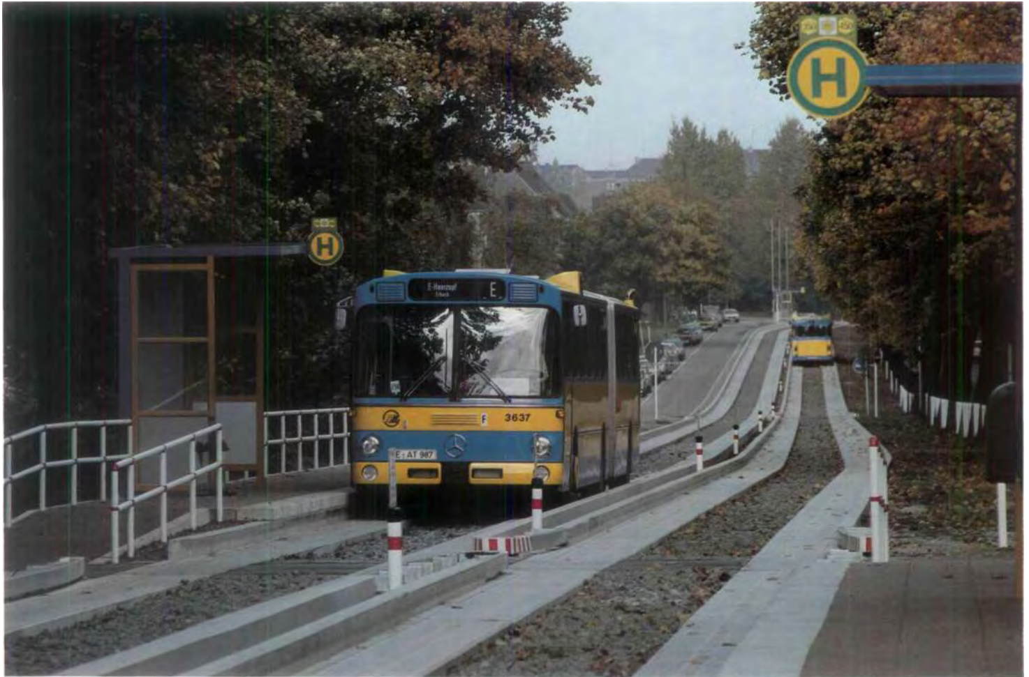
Introduction of the first Mercedes-Benz track-guided bus line in Essen. 21 Mercedes-Benz articulated pusher buses model O 305 G are in operation.
