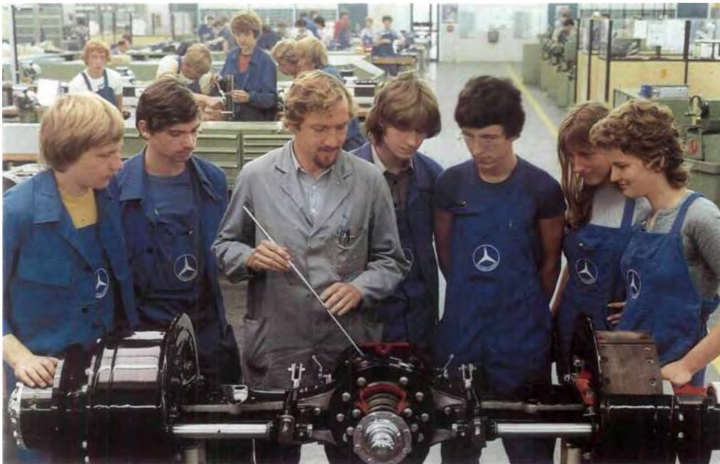
On-the-job-training at the Kassel axle plant. Sectional model of a truck rear axle.
