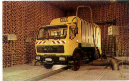
Municipal vehicles in the noise test stand facility (left). Electronic measuring and recording devices for noise tests (below).
