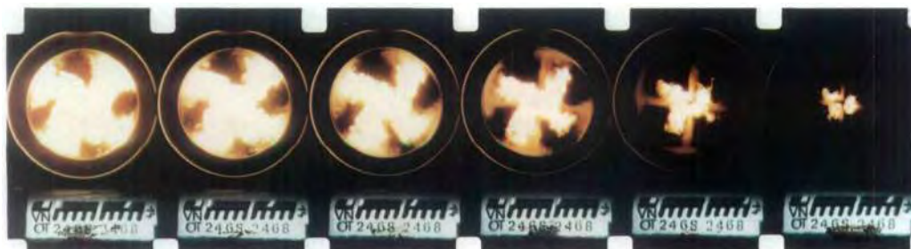
High speed photography is used for recording mixture formation, flame development and air intake in diesel engines.
