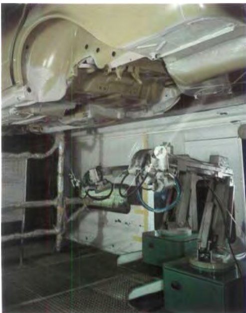
Relief from heavy manual work. In the Sindelfingen car plant, industrial robots spray PVC undercarriage protection.
