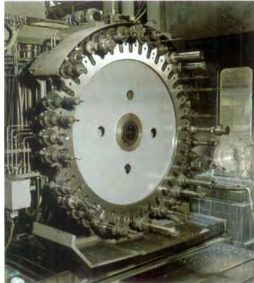
Automatic change installation for 30 different tools. Computer-operated processing center for commercial vehicle automatic transmissions at the sub-plant Rastatt of the Gaggenau plant.
